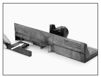
Figure 13. Installing the pocket jointing fence.
